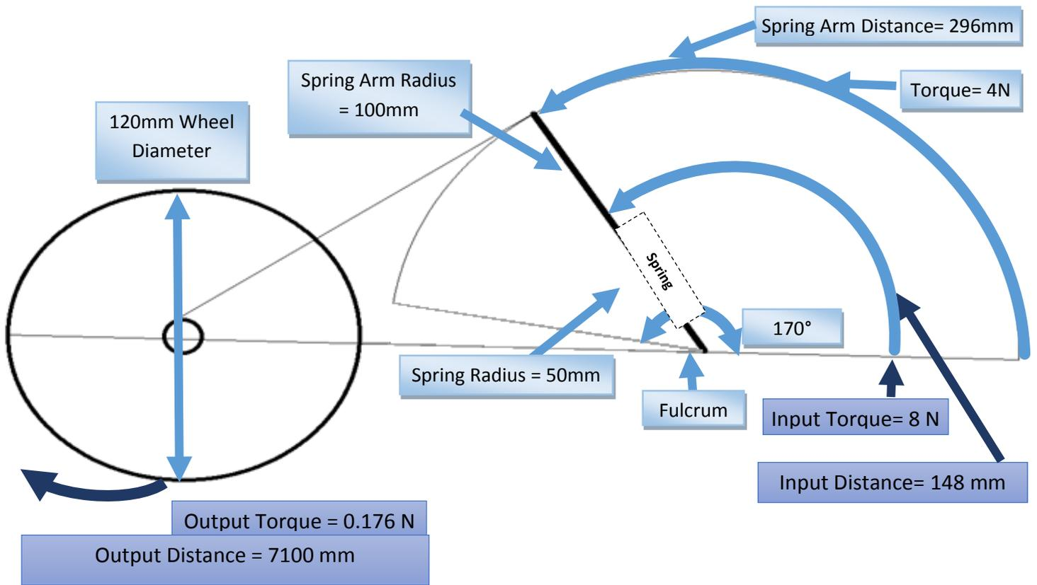
$$\text{Mechanical Advantage (MA)} = \frac{\text{Input Distance}}{\text{Output Distance}}$$
