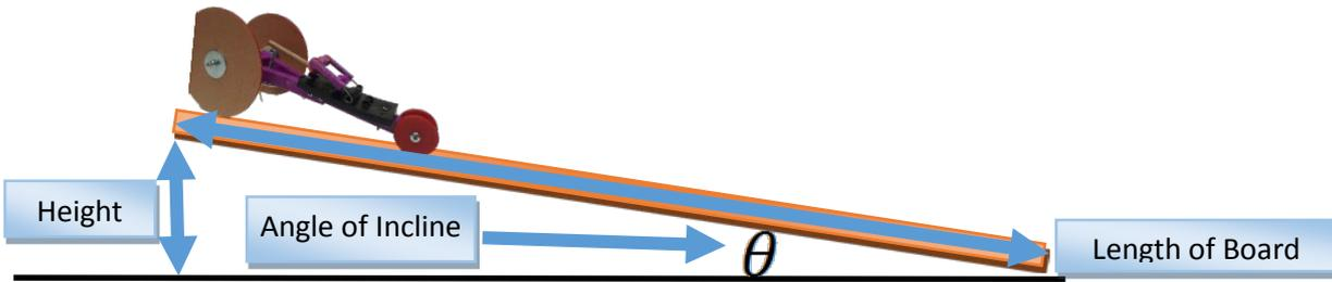
1. Calculate Angle of Incline by using  $\sin(\theta) = \frac{\text{Opposite}}{\text{Hypotenuse}}$
