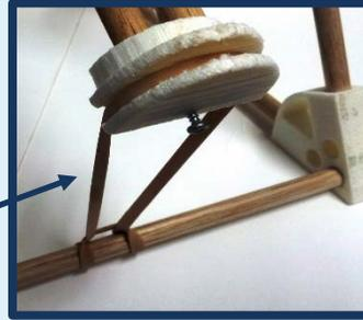
**Results:** The greatest projectile displacement was produced with the maximum launch power using three parallel rubber bands (Table 3 & Fig. 3).
