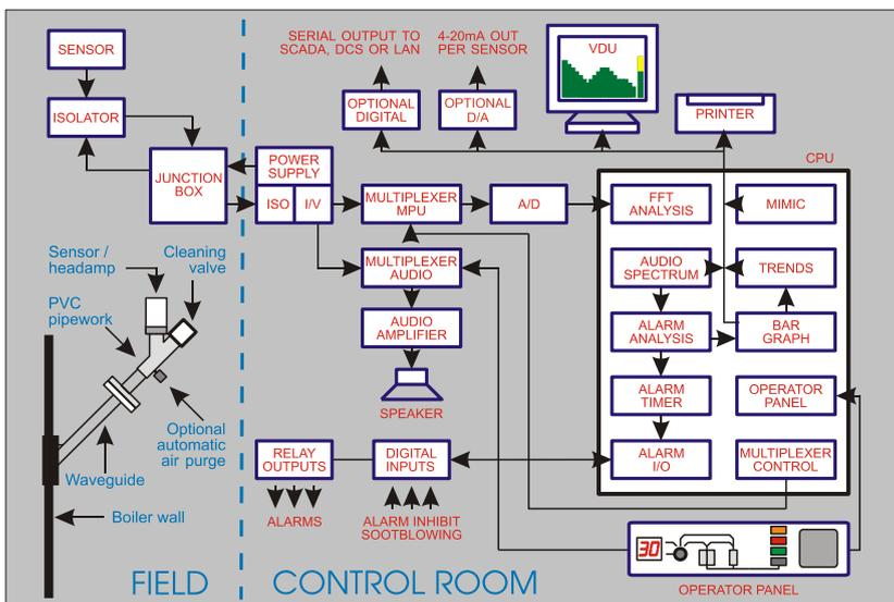
**Audio** allows operators to listen to the sound inside the boiler at any sensor point by selecting the required channel. The audio sound is heard through the speaker built into the multiplexer operator panel.
