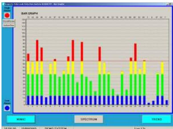
**Bar graph** mode has provision to display up to 32 processed sensor alarm signals simultaneously on the monitor. The vertical coordinate is the present alarm level and the horizontal is the sensor number. Under tube leak conditions, the graph climbs from the normal Green zone, to Yellow for caution, and to Red to show a critical situation has been reached. Fault Conditions and Low Sensor Levels are displayed in Blue.
